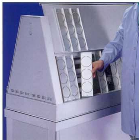
Test specimens are mounted in convenient snap-ring holders.
