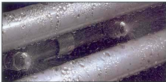
All models of QUV use condensing humidity to simulate the effects of rain and dew on your specimens. In addition, the QUV/spray allows direct water spray for thermal shock and erosion.
